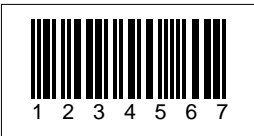
Interleaved 2 of 5 + CHECKSUM
